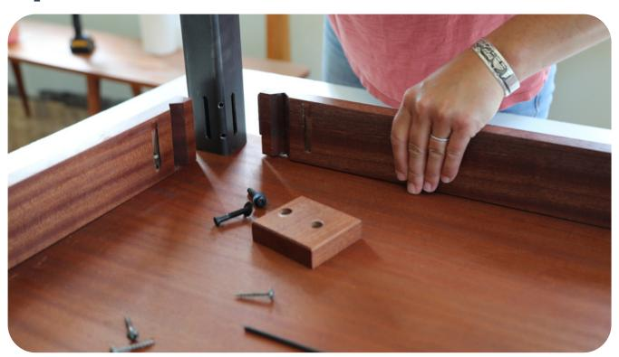
3: Place Block & Bolts. Using the supplied wrench, tighten each bolt until it stops turning and the handle begins to spring back. Repeat for each remaining leg.
